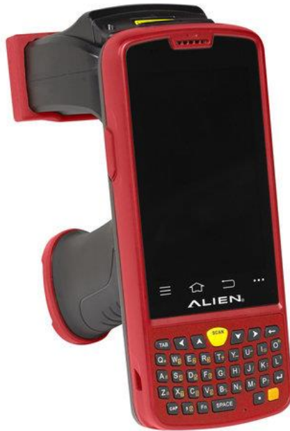
fig. 13 – Alien ALR-H450 Handheld RFID reader [41]
