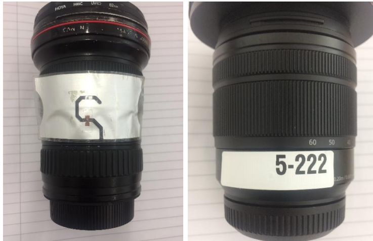
fig. 27 – (left) - Lens 2 with tag 3 - Canon EF 16-35mm f/2.8L III USM; the radius is 41.5 mm
