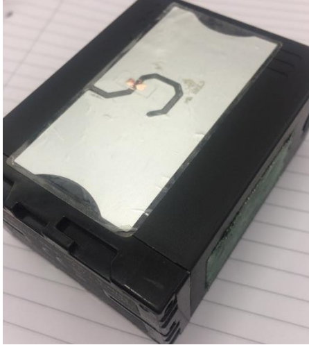
fig. 25 – (left) – 3 Avery Dennison AD-550M5 tag stuck on the NP-F970 battery pack
